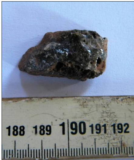
Figure 5.20: Crucible with flecks of gold remaining in it. Found at the Barrier Hut.
