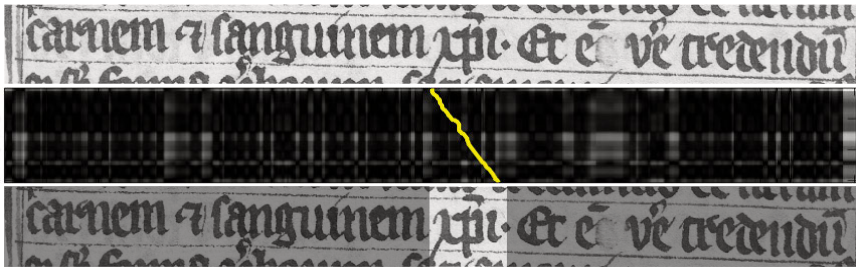
Figure 3.8. An example of a warping path “cutting” through a full text line, using dynamic time warping (section 3.3.1). The cost matrix, i.e. element wise differences between feature vectors, is shown in gray scale in the background with the warping path in colour.
