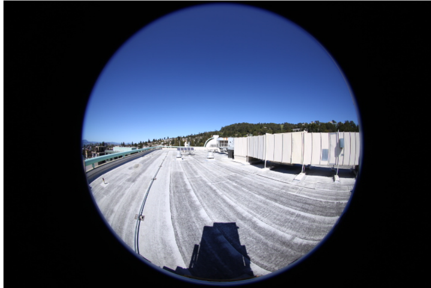
Figure 6.22: The properly exposed LDRI from the LDRI^{11} showing the directly orthogonal CUBE 2.0 shadow from the CFS test aperture.
