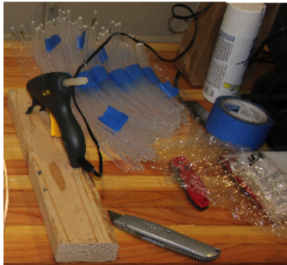
Figure E.19: The uncut \frac{1}{4} " diameter, poly(methyl methacrylate) (PMMA) optical fibers.
