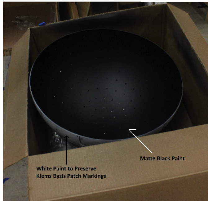
Figure E.17: White then matte black paint coats the inside of the acrylic hemisphere.
