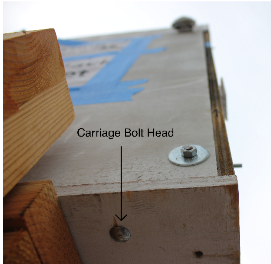
Figure E.39: Carriage bolt heads extending from the bottom of the CUBE 2.0. These steel “dishes” of sorts allow for low friction sliding of the CUBE 2.0 system.
