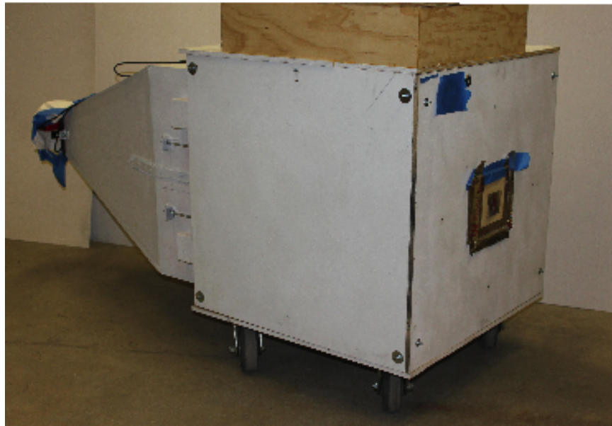
Figure 4.13: The complete enclosure of the CUBE 2.0 system with the measurement cone installed.
