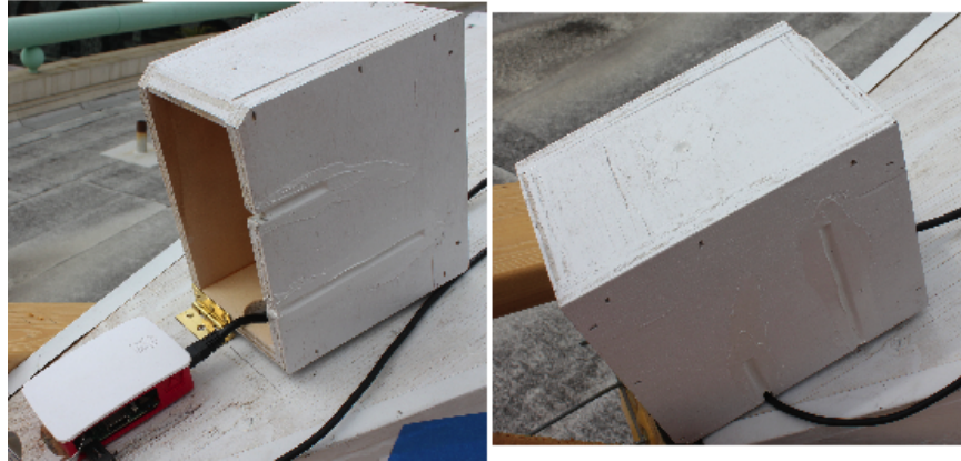
Figure E.37: Enclosure for the RPiCM as to protect it from the elements.
