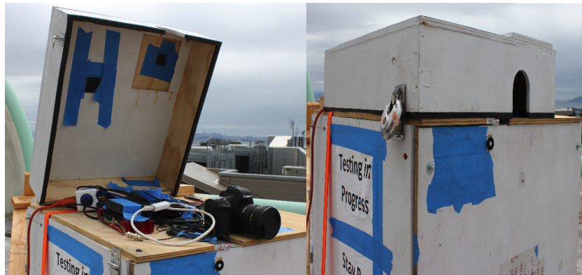
Figure E.36: The second enclosure for the Canon 6D, MacBook Pro, Ethernet Router, USB connector, Power Hub.
