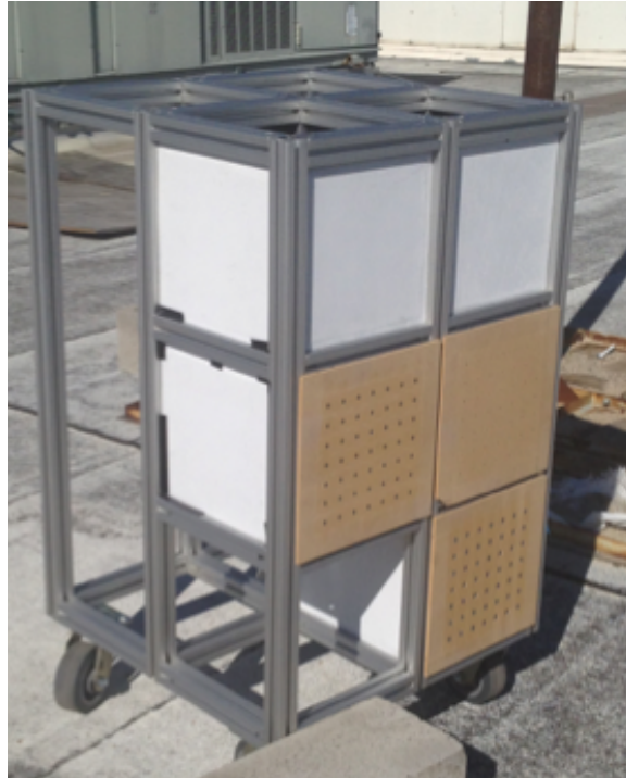
Figure 4.1: CUBE 1.0 which uses the transmission method to investigate building envelope panels.
