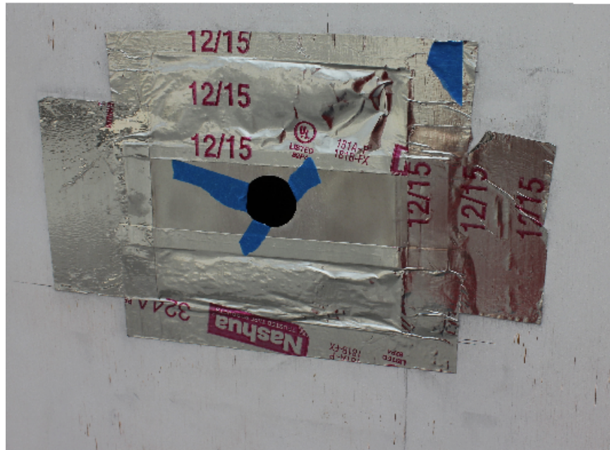
Figure E.31: Brass CFS holder in place on CUBE 2.0. The 1 inch hole is the CFS test aperture.
