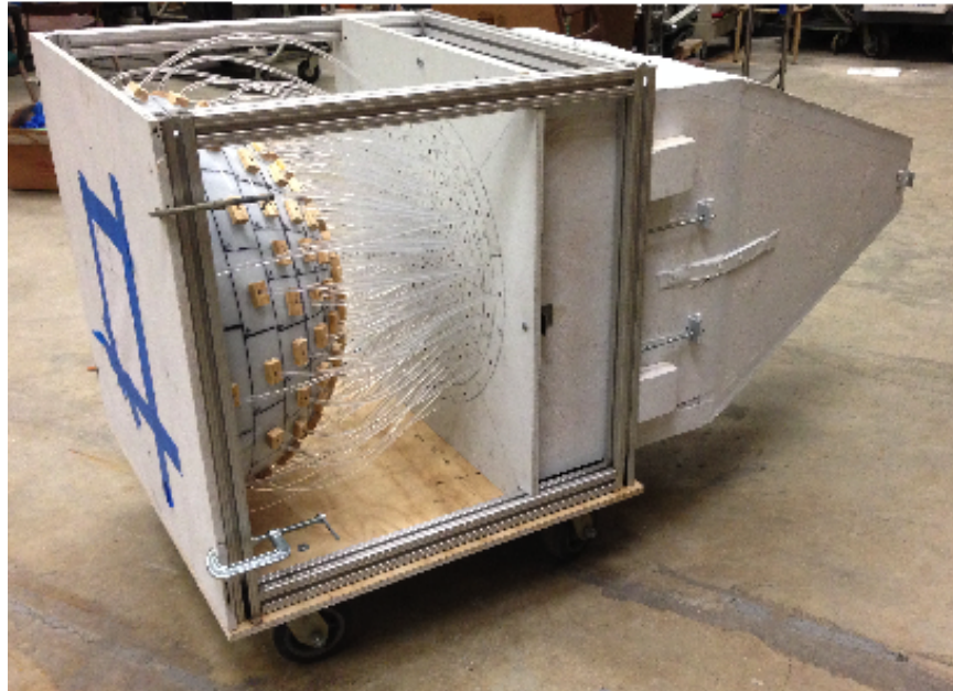
Figure 4.14: The total optical fiber sampling system from exiting luminance measurement hemisphere holding the “sampling” optical fiber end, through optical fiber “measurement” end terminating at the measurement cone .
