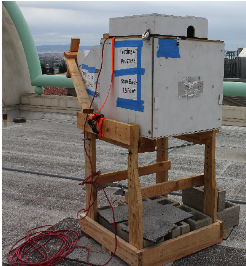
Figure E.40: CUBE 2.0 support frame, which is permanently deployed on the roof of Cory Hall at the University of California, Berkeley.
