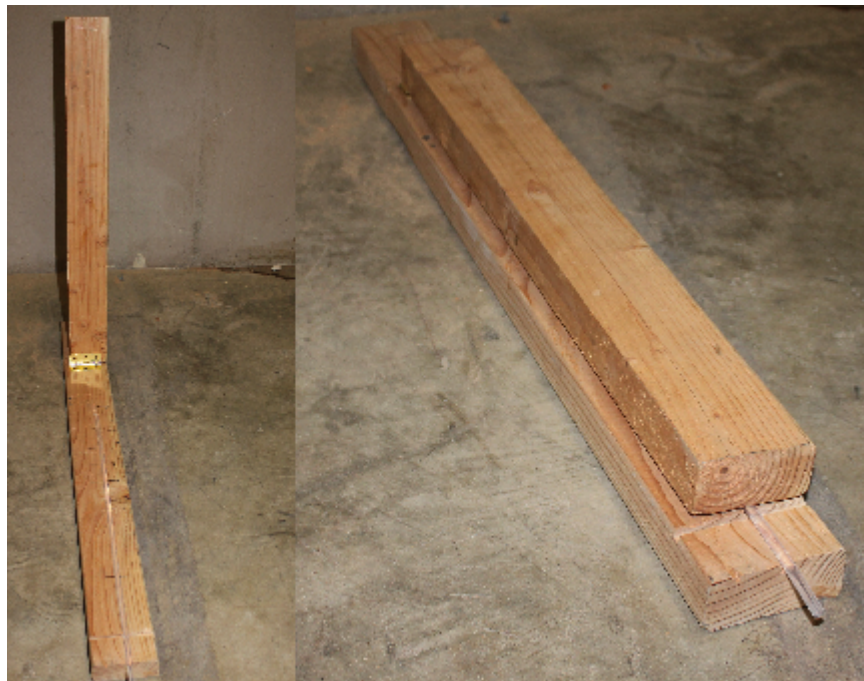
Figure E.20: A simple 2×4 cutting device used to ensure consistent optical fiber length.
