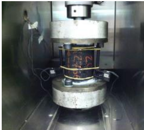
Figure 3.7 – Specimen prepared for tension-compression test (Nascimento et al., 2014)
