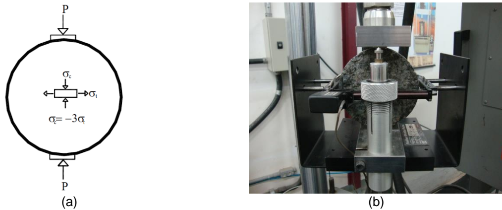
Figure 3.4 – Indirect tensile test: (a) stresses during the test and (b) equipment commonly used
