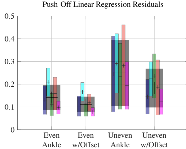
Figure 4.6: Root mean square (RMS) of the residuals from the linear regression performed for torque versus ankle angle and ankle angle with offset, respectively, for Eq. 4.4 (during push-off) for healthy subjects.
