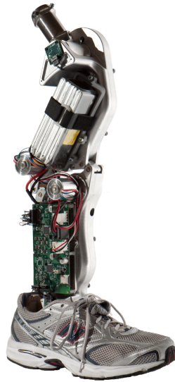
Figure 1.1: Generation 2 Vanderbilt powered knee and ankle prosthesis prototype.
