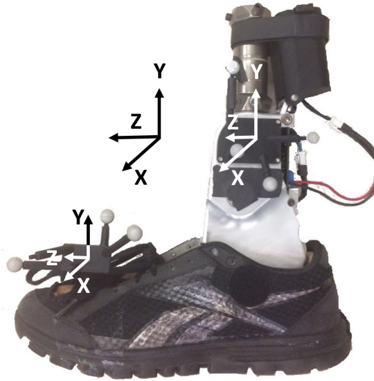
Figure 4.10: Gen 3.2 prosthesis experimental setup and axis convention.
