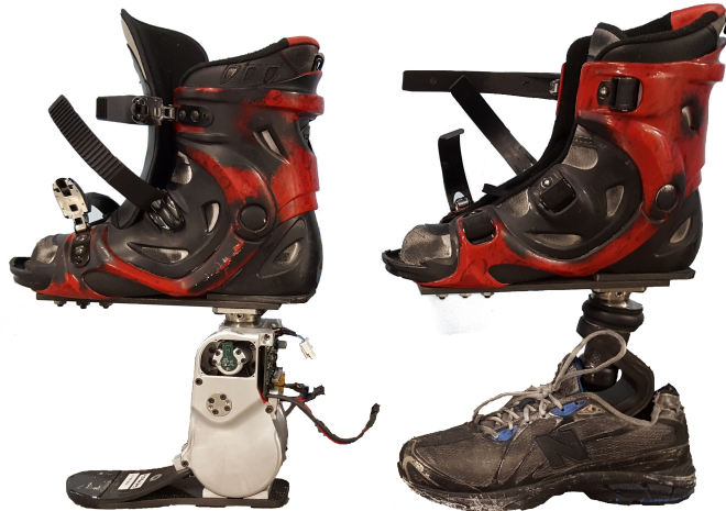
Figure 1.3: Sample able bodied adaptor setup for powered and passive ankle prostheses.
