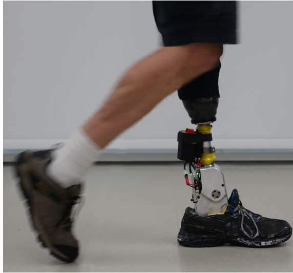
Figure 4.7: Amputee subject walking with Vanderbilt powered ankle prosthesis prototype.
