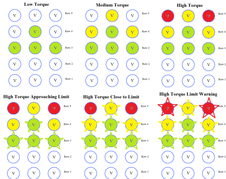
Figure 5: Torque-dominant model examples in the extension direction with the top row showing torque within a normal range (green-yellow-red color transition used to show increasing torque intensity) while the bottom row shows how torque approaching the torque limit will lead to an increase in the number of factors pulsing (identified by jagged edges around the factor).
