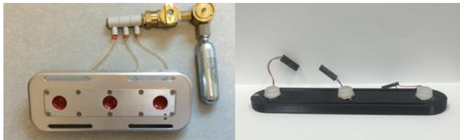
Figure 8: (Left) Quasi-static pressure feedback array. (Right) Vibrotactile array.
