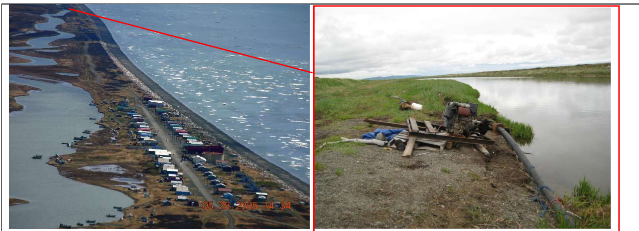
Figure 1.3 Shaktoolik: Concerns about drinking water quality. View of town (left) and water intake infrastructure, first bend, Tagoomenick River (right). There is a concern about saline intrusion into the drinking water supply as the waves are able to reach the river, that supplies the town's drinking water. Credit: USACE, BEA, 2009 (picture left), LEM 2013 (picture right)
