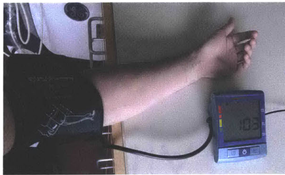
Figure 4-1: Photo of one of the oscillometric cuffs used in this work. After pressing the start button on the device, it automatically inflates and deflates, then it reports the blood pressure.
