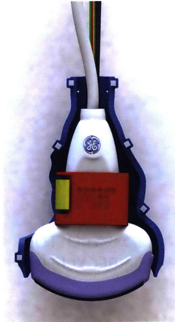
Figure 4-7: Solid modeling mock-up of the force measurement attachment used during this dissertation. The red clamp is attached to the blue outer clam shell through a load cell. Note that while the image shows a curved probe, only linear probes were used in this dissertation. The device was developed by Dr. Matthew Gilbertson and Athena Huang.
