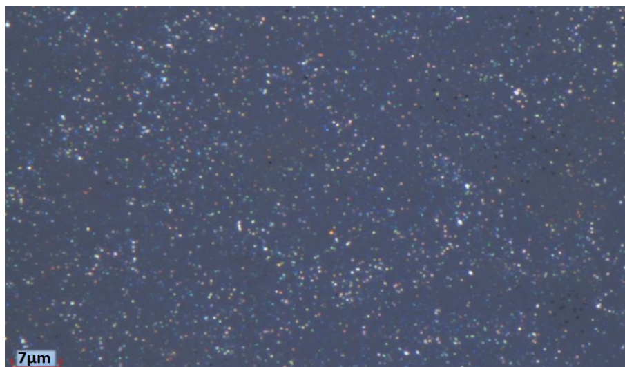
Figure 3-5. Optical microscope image of coated glass sample (100X magnification).
