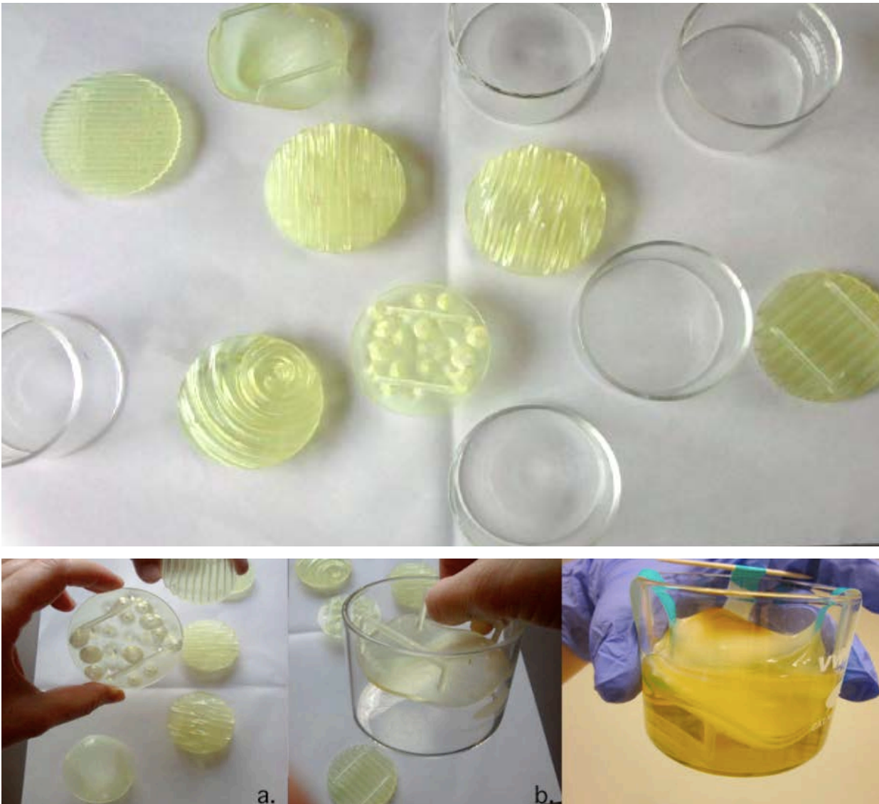
Figure 3.4.9: Molding bacterial cellulose biofilm as it grows on 3D printed molds and introducing texture (with S.Araya).
