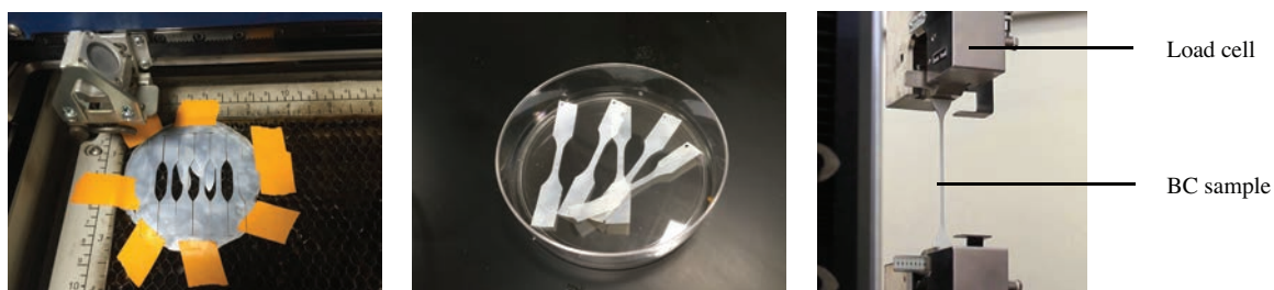
Figure 3.4.8: Lasercutting bacterial cellulose samples for tensile testing (with M.Gazit)..
