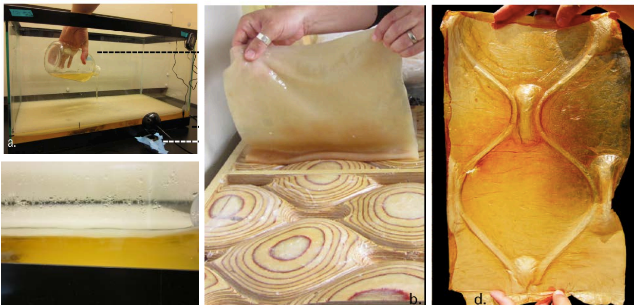
Figure 3.4.10: Molding bacterial cellulose biofilm post- grows on CNC-milled mold (with S.Araya).
