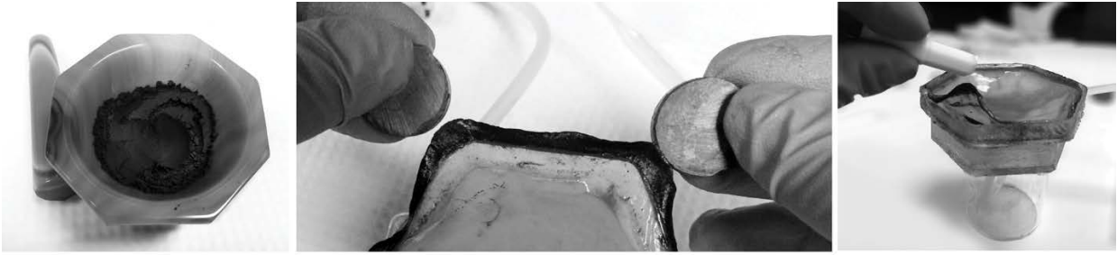
Figure 3.4.5: A composite of bacterial cellulose and Magnetite (with M.Gazit)..
