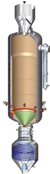
Figure 3 Example for fixed-bed gasification - BGL gasifier , adapted from Hirschfelder [56]
