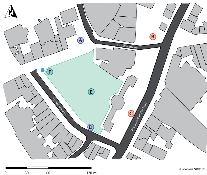
Fig. 5: Research site Elisenbrunnen in Aachen, including depicted measurement locations A–F (colored circles). The park area is marked with a green color field, whereas the light blue color field represents a water body. Gray areas depict buildings and black areas represent traffic arterials. Reworked after journal paper I.
