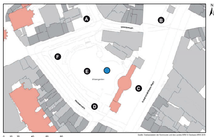
Fig. 2. Map of the research site with marked monitoring locations (A-F) where measurements with the OPC were carried out (black dots) and marked location where meteorological measurements as inflow boundary conditions for the model were conducted (blue dot).
