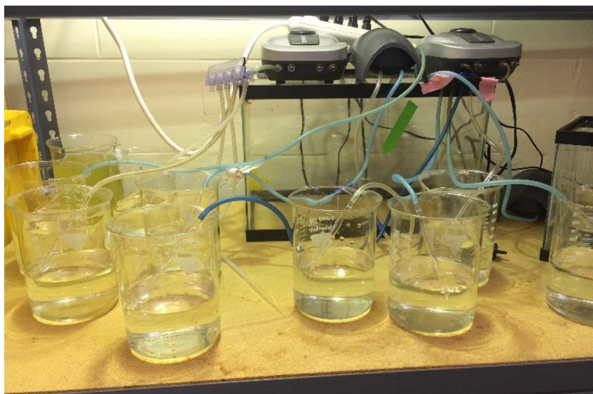
Figure S1- (a) Glass vials containing algae cells, media, and PCB-impregnated polymer, (b) glass carboy containing, Daphnia media, and PCB-impregnated polymer, (c) replicate Daphnia exposure beakers.
