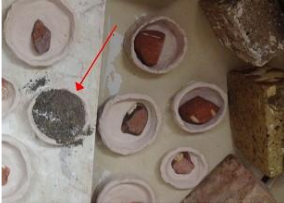
Photo 6.18. Image of samples from Firing Test #4 showing the samples in place within the kiln directly after firing, note the red arrow is pointing to a coarse-grained igneous rock that exploded during firing. Right: The same sample that exploded pictured with another thick section and the original cobble that the sections were cut from.
