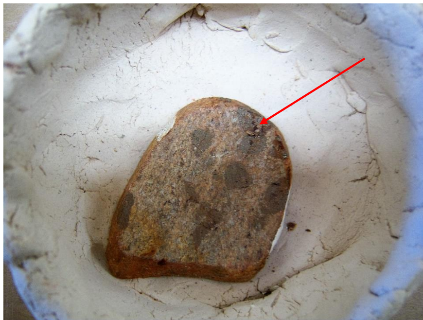
Photo 6.17. Sample from Firing Test #3, showing a large stress fracture (red arrow) and reddening.
