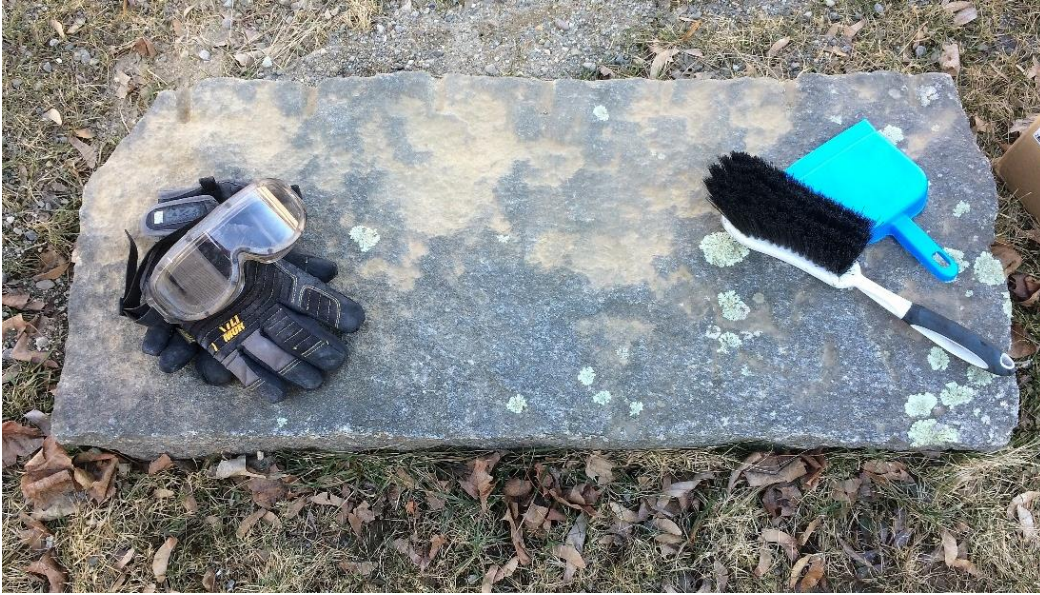
Photo 6.25. The mechanical pressure tests were conducted on a large piece of cut granite with an unmodified granite hammerstone, safety equipment, and a small hand broom for cleanup. All tests were video recorded using an iPhone 6.
