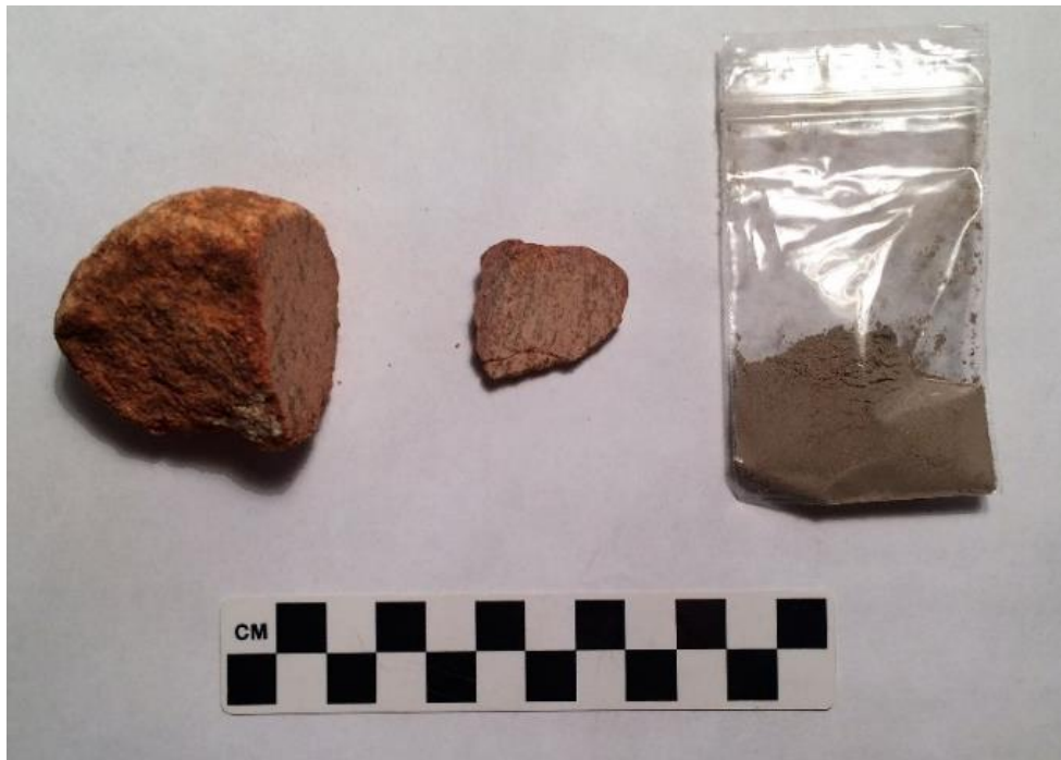
Photos 6.19. The same sample that exploded during Firing Test #4 pictured with another thick section and the original cobble that both of the sections were cut from.
