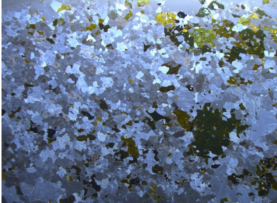
Photo 6.13. Low magnification (7.5x) of the same biotite granite from Sinking Ponds, as shown in Photos 6.10-6.11. Note the green biotite and clear-colored felsic minerals (mostly quartz and feldspar).
