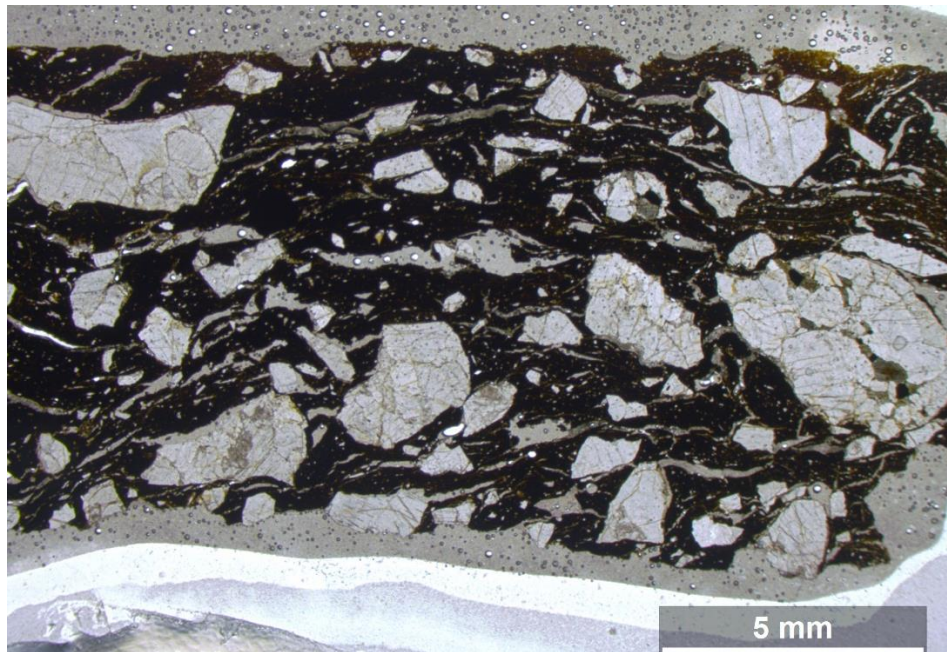
Photo 5.3. Low-power magnification of crushed rock inclusions from Portage Vessel 1, Body Sherd 1. Note that none of the crushed rock inclusions occur in sizes smaller than 0.25 mm in diameter and have angular to very angular edges. Image taken at 5x in plain polarized light.
