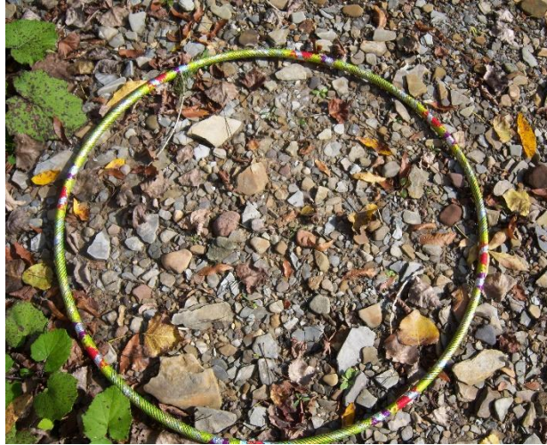
Photo 6.2. The Hula Hoop used to collect random rock samples during the glacial distribution study. Note the hoop measures 1.067 m (42 in) in diameter and all cobbles laying inside the hoop were collected each time it was thrown, until all 100 cobbles were gathered.
