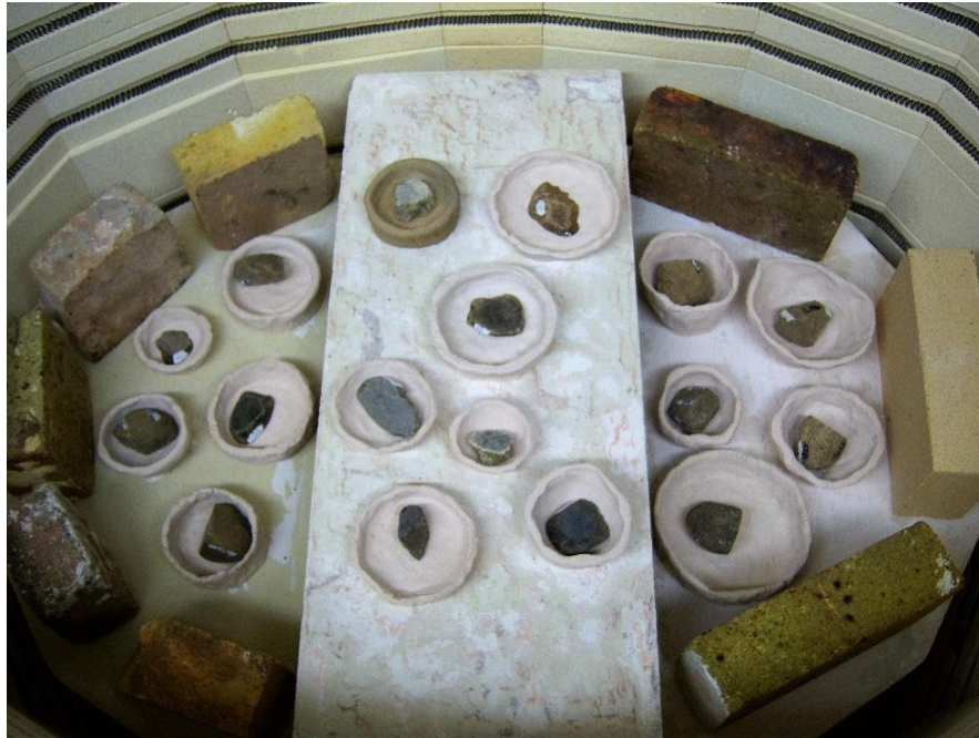
Photo 6.16. Image of the Bartlett kiln prepped for firing. Brick was placed around the edges of the kiln to protect it in the event that samples exploded during firing. The samples were kept spaced apart to avoid them melting together.
