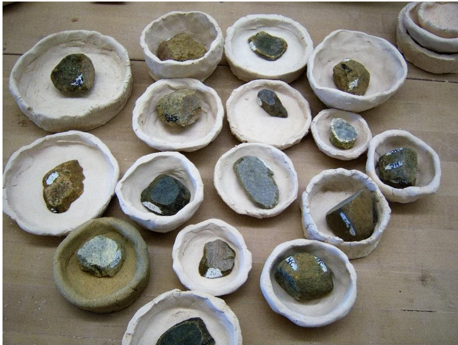
Photo 6.15. Image of a round of samples prepared for firing. Prior to firing, 100 round ceramic stoneware ramekins were produced by the author in order to hold samples during firing. Each ramekin was incised with a number on the bottom corresponding to the sample information. Samples were also labeled with whiteout and a sharpie, but all the labels melting off during firing.
