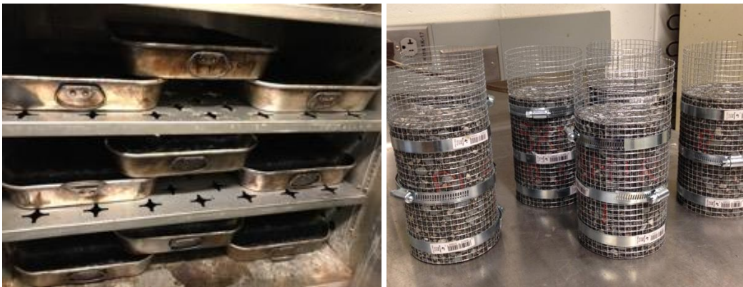
Figure 6-1. Aging of compacted specimens (right), and loose mix asphalt (left)
