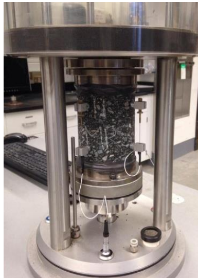
Figure 2-7. Uniaxial Direct Tension Test Configuration
