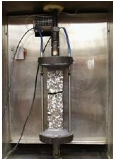
Figure 2-8. TSRST Test Configuration (Asphalt Research Consortium, 2007)
