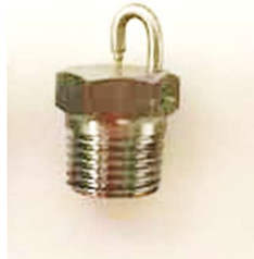
Figure 6-4 Spray nozzles 1/8 PJ20 used for this study
