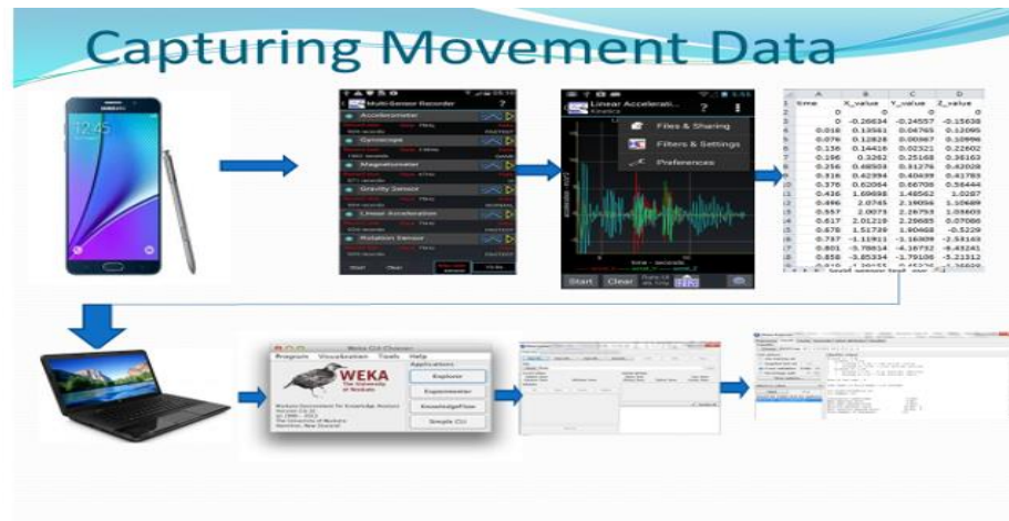
Figure 3.18 Process: Complete Capture and Evaluation of the Data from Motions
