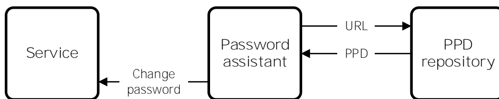
Figure 7.1: Data flow of the automatic password change procedure.
