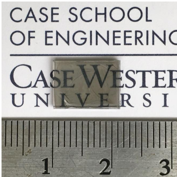
Figure 5.2 Photo of transparent MoS 2 -3DG thin film on PDMS.
