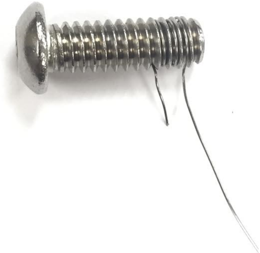
Figure 7.4. A Kanthal A-1 wire turned into shape in the threads of a 1/4-20" bolt.
