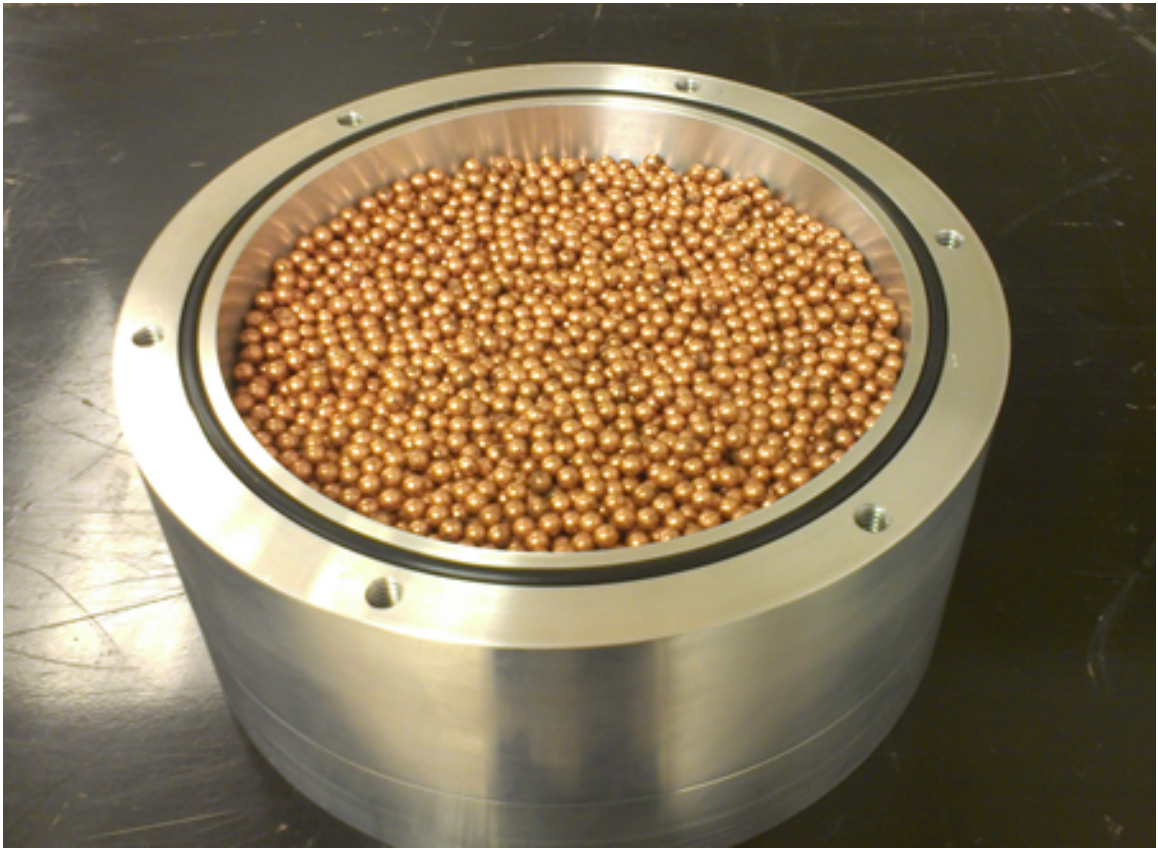
Figure 4.6. Copper BBs are packed above the screen to create a large pressure drop to encourage mixing and smooth flow.
