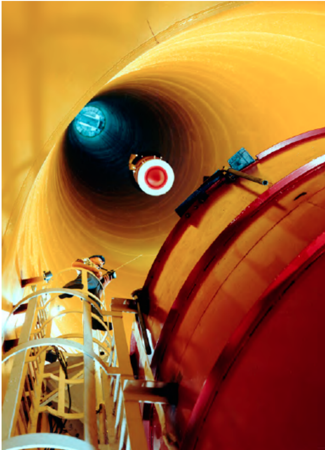
Figure 6.1. A Stock photograph of the NASA Zero Gravity Research Facility vacuum drop shaft. The decelerator is shown in red on the right. In the center a drop vehicle is being recovered with a crane from above. [NASA Stock Photo GPN-2000-001454, 1966]
