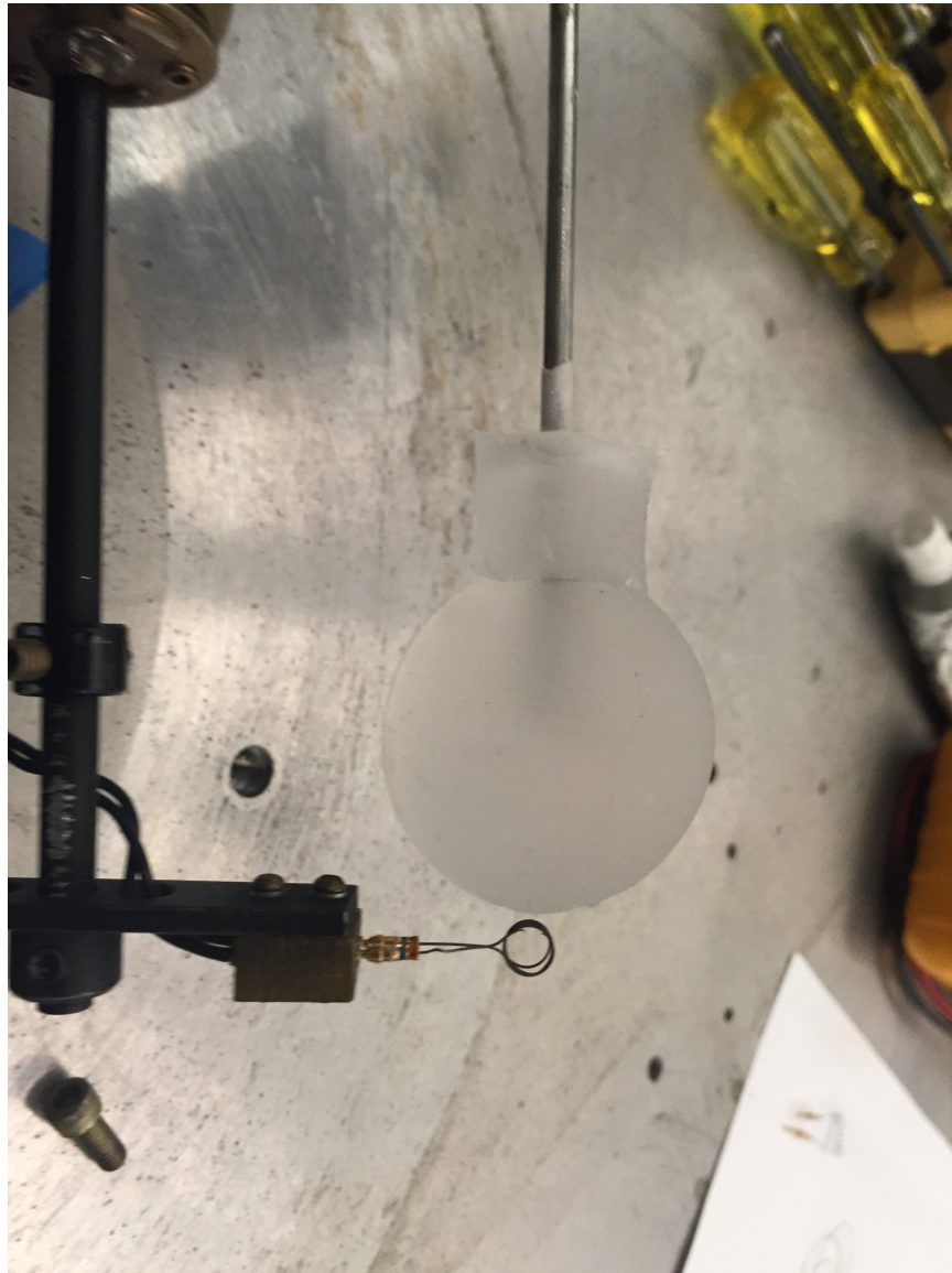
Figure 6.3. Igniter configuration for GEL testing in the ZGRF
