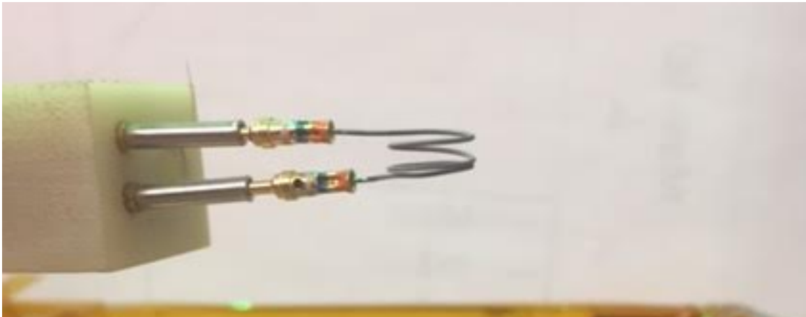
Figure 7.8. A 27 AWG Kanthal A-1 coil igniter which has survived 100 thermal cycles.
