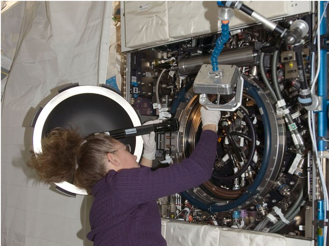
Figure 7.1. Astronaut Sandra Magnus installing an experiment module into the Combustion Integrated Rack aboard ISS (Stock NASA Image ISS018E35752)
