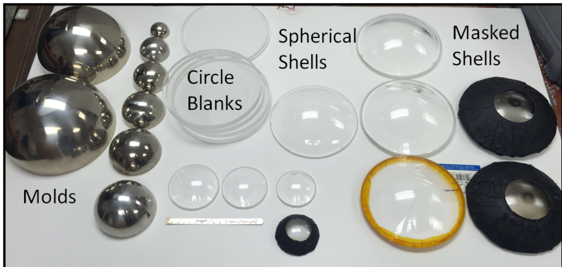
Figure 3.1. The components for making spherical PMMA shells. From left to right, the various sized spherical molds, circular PMMA disks, shaped PMMA spherical shells, and masked shells with controlled exposed surface area.
