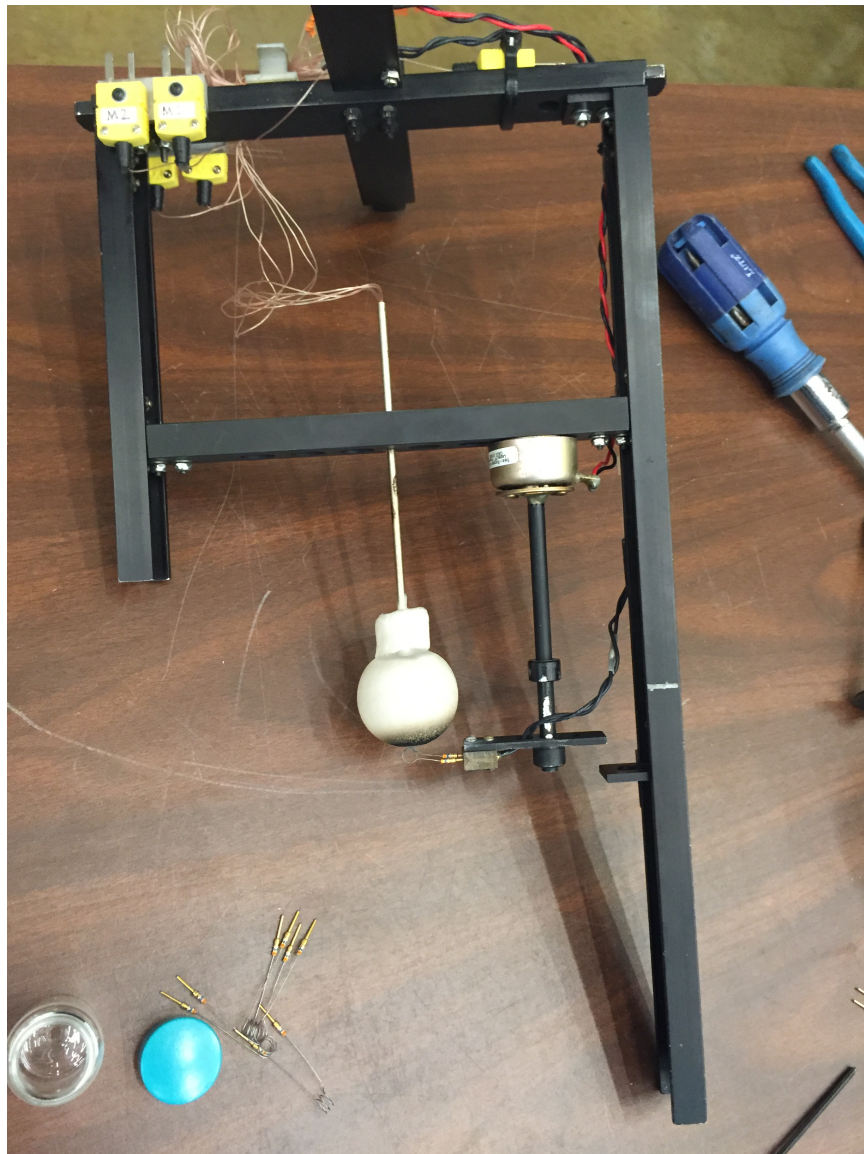
Figure 6.4. Combustion Tunnel sample holder modified for use with the GEL sphere samples
