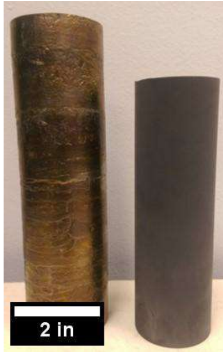
Figure 2.1: As-cast (left) billet was approximately 2 inches in diameter x 1 feet long while HIPed (right) and machined billet was approximately 1.77 inches diameter x 1 feet long. The as-cast sub-scale billet was removed from the original 10 feet x 2 inch diameter cast billet.
