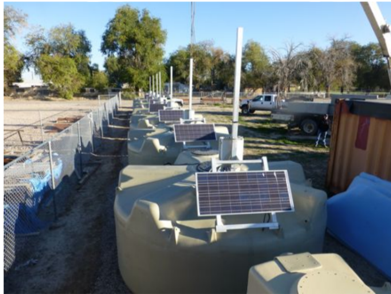
Figure 7.4: Top: Proposed co-location sites for the AN WCDs. Bottom: Photo of the staging area showing the AN stations available for deployment.
