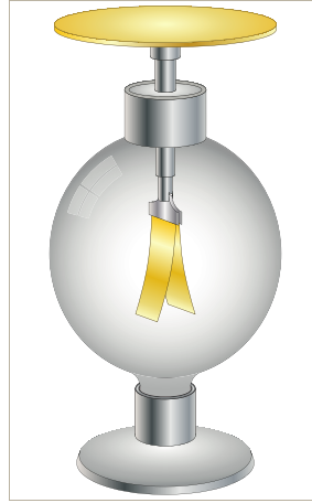
Figure 1.1: Artist's depiction of a late 18th century electrostatic apparatus. This model uses gold foils secluded in a glass jar to prevent air currents, moisture and other externalities from disturbing observations. To measure charge the experimenter holds the object close to the top disk which inductively charges the apparatus. The gold foil leaves will be displaced according to the charge magnitude.
