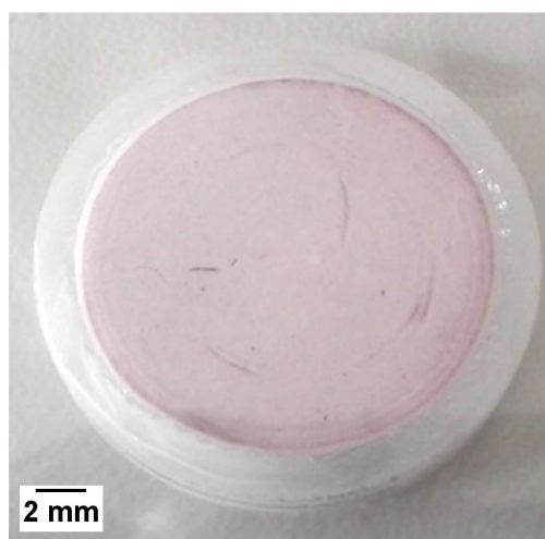
Figure 4.46 Top view optical image of P5 frit after loading of with Au@SiO 2 yolk-shell nanoparticles.
