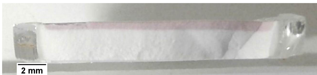
Figure 4.48 Cross-sectional optical image of P5 frit. The upper pink part shows the loaded Au@SiO 2 particles and the lower white part show the empty frit.
