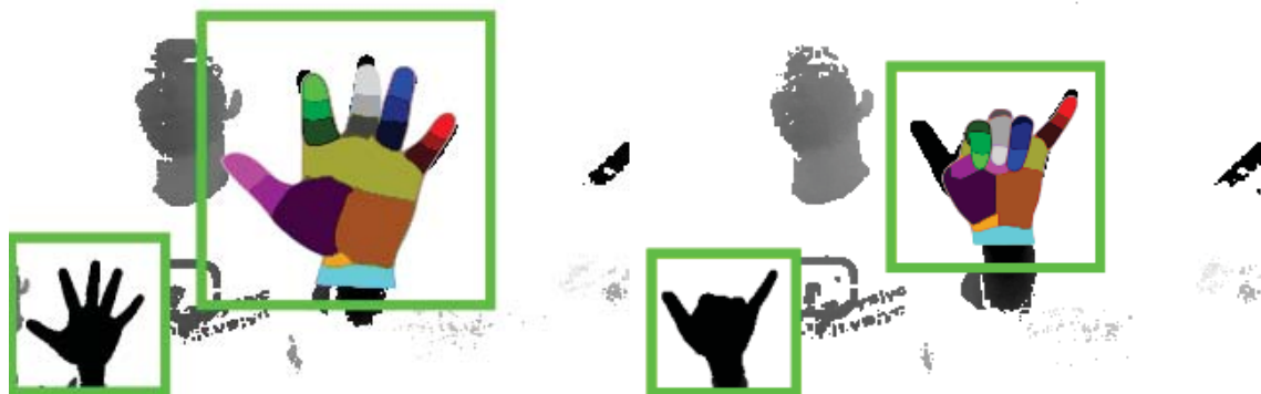
Figure 2.13: Min versus max error: Compared to state-of-the-art, our 1-NN baseline often does relatively better under the average-error criterion than under the max-error criterion. When it can find (nearly) an exact match between training and test data (left) it obtains very low error. However, it does not generalize well to unseen poses (right). When presented with a new pose it will often place some fingers perfectly but others totally wrong. The result is a reasonable mean error but a high max error.
