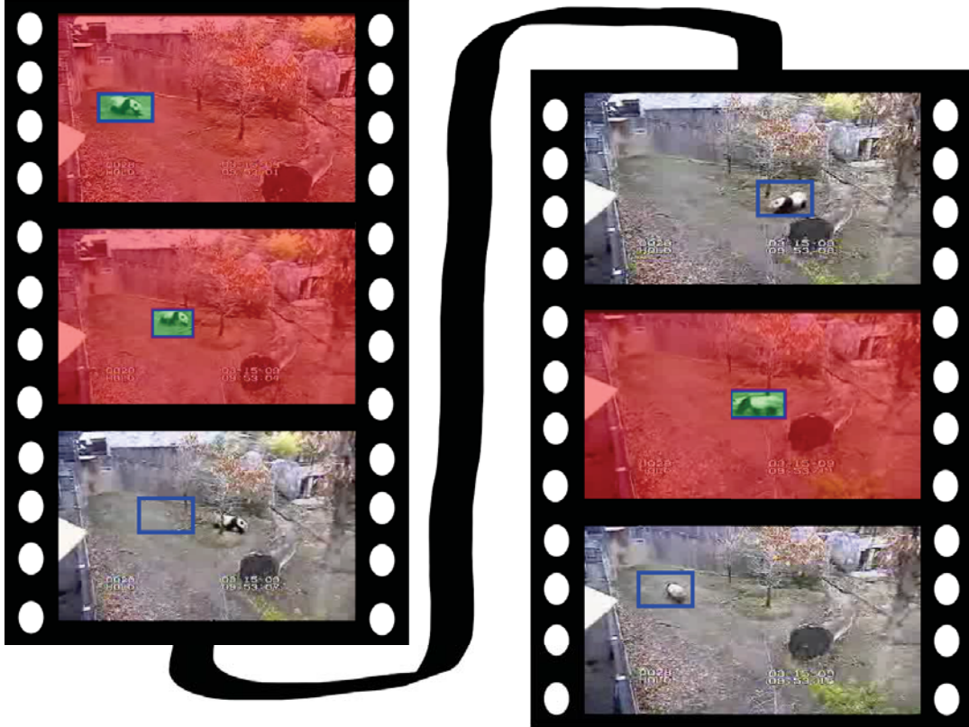
Figure 5.1: Our tracker uses self-paced learning to select reliable frames from which to extract additional training data as it progresses (shown in red ). We use such frames to define both positive examples and a very-large set of negative examples (all windows that do not overlap each positive). By re-learning a model with this additional data, and re-tracking with that model, one can correct the errors shown above. We show that it is crucial to revisit old frames when adding training data; in terms of self-paced learning, a concept (frame) that initially looks hard may become easy in hindsight.
