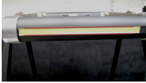
FIGURE B.7: Red lines are drawn in to show where the epoxy should be dribbled onto the curved edge of the rotatable plate
