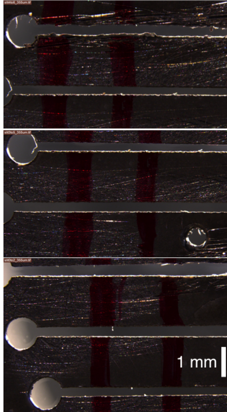
FIGURE 3.12: Microscope image of Cd mask with 1 mm scale used in Section 3.1.8. The image is a composite of three microscopy images.
