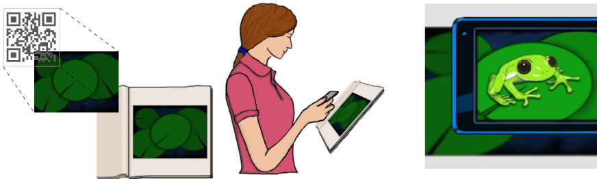
Fig. 4. The watermark, here resembling a two-dimensional barcode, is embedded in the image which is then printed. The user can read the watermark with a camera phone and the content is shown according to the watermark information. Here, an augmented reality application is launched in which the application launches a view according to the watermark, in this case, an animation of a frog.
